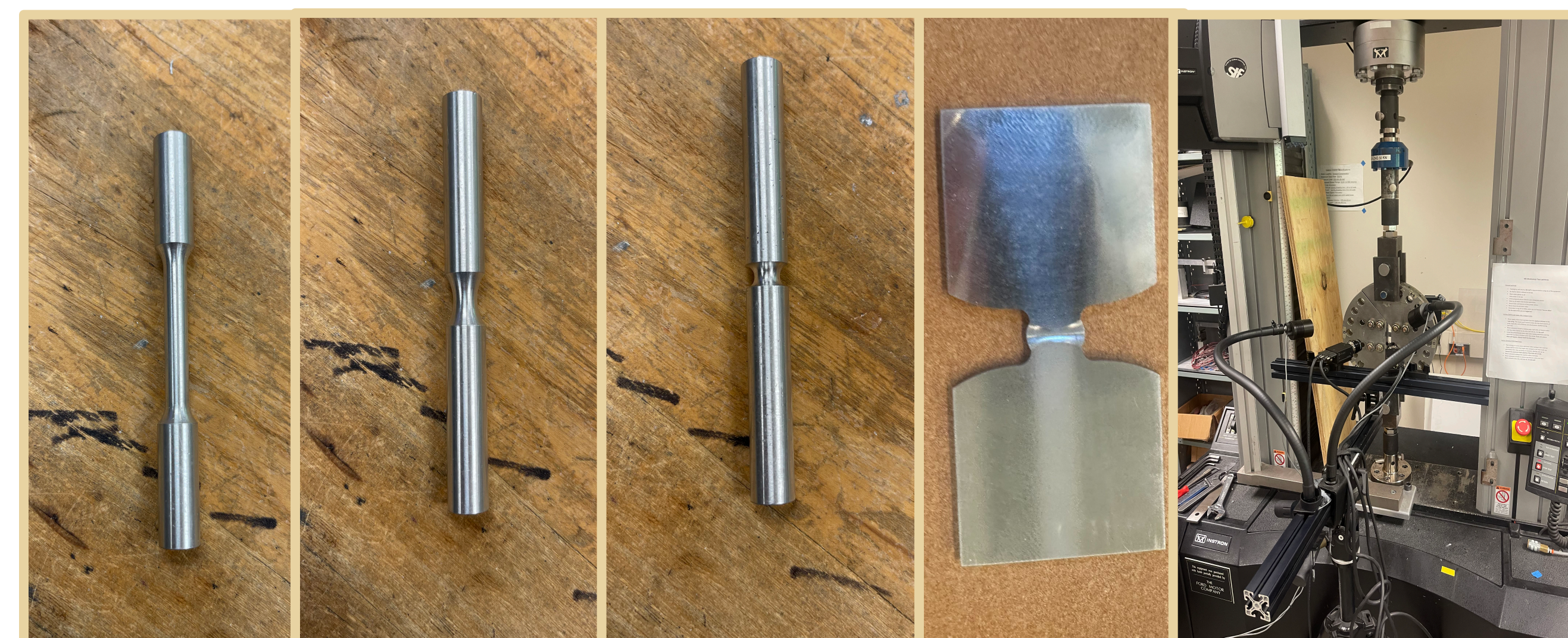
Left to right: Long Round Bar, Large Notch Round Bar, Small Notch Round Bar, Butterfly Specimen, Instron and Arcan fixture with 3D DIC
